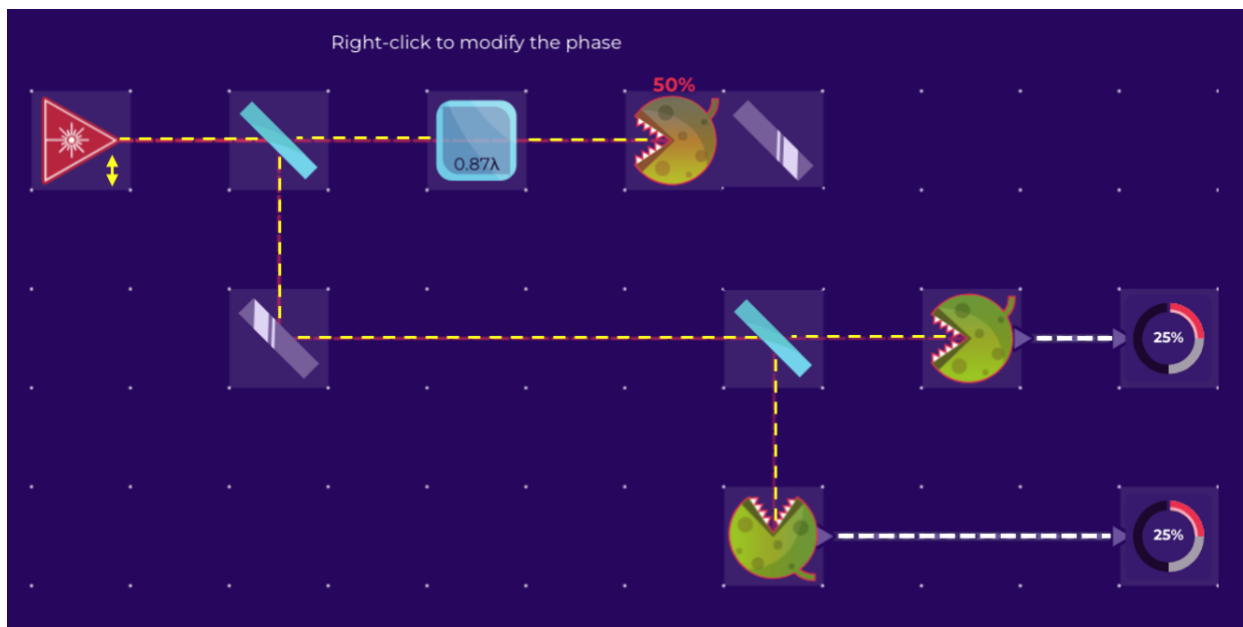
Figure 27. Before interference we measure the same values for probabilities as in the classical case. If we remove the detector in the top arm of the MZI we obtain the situation from Figure 26.
