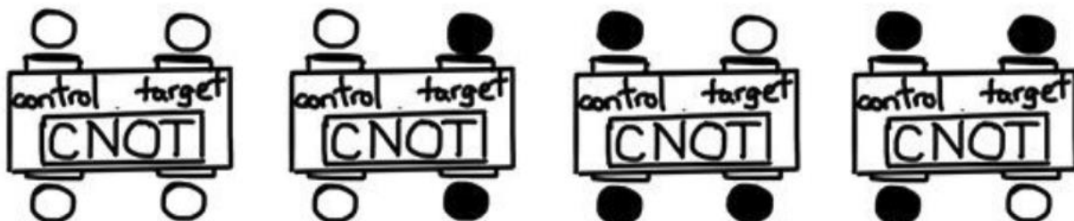
Figure 3. Behavior of the two qubit gate C-NOT.
