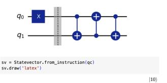
circuit is equivalent to a SWAP so if  $q_0 = q_1 = |0\rangle$  then after the NOT gate the state is  $|10\rangle$  which means that at the end, after the three C-NOT gates will have performed their intended functions the state should be  $|01\rangle$ . Yet Qiskit reports the final state as  $|10\rangle$  Is there a mistake somewhere?
