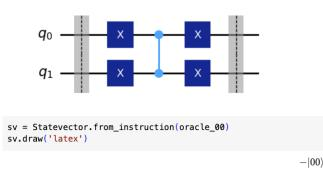
We know that the controlled-Z (C-Z) gate adds a phase only when both qubits are  $\bigcirc$ . That should be enough to realize why this is indeed the oracle for  $\bigcirc$ : any other state would fail to produce the needed prerequisite for an added phase. It is now easy to determine the other three oracles:
