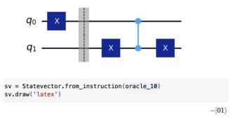
First off we note again, here, that the name of the quantum oracle (circuit) is chosen with the traditional numbering convention of qubits in mind (i.e.,  $q_0$  first, then  $q_1$ ) whereas the reporting is done using Qiskit numbering convention, that is,  $q_1$  is listed first, then  $q_0$ . Then the state that is identified by the oracle, in Qiskit, as the solution, is consistent with  $\bigcirc$ .
