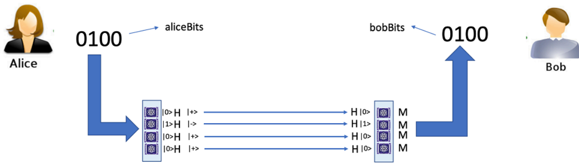
Figure 8.12 Alice applies a Hadamard gate before sending a qubit, Bob applies a Hadamard gate before measuring the qubit.
