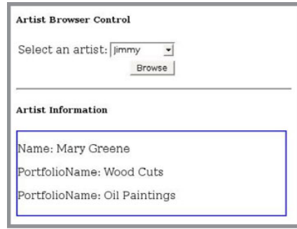
Figure 8.3 Our artist browser submits Ajax requests to the web application and receives JSON responses via our custom JSONResult .
