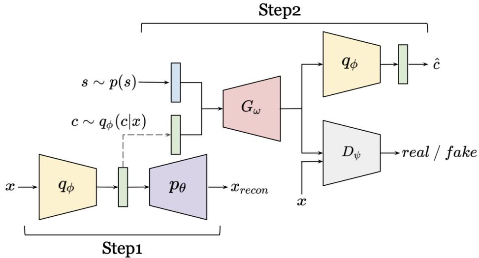
Figure 2.1: The ID-GAN network. The  $\beta$ -VAE model is trained in Step1. Then the latent space of the trained  $\beta$ -VAE model is concatenated with the noise vector as input to the generator, and the GAN module is trained. The variable  $s$  in this figure is written as  $z$  in the equations above. The schematic was taken from (Lee et al. 2020).
