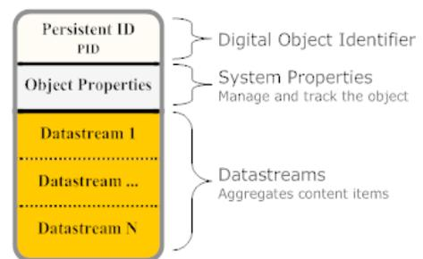
Fig. 3 Fedora Digital Object Model
