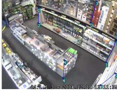
Figure 3: VZ can be found by manually marking two or more vertical straight lines
