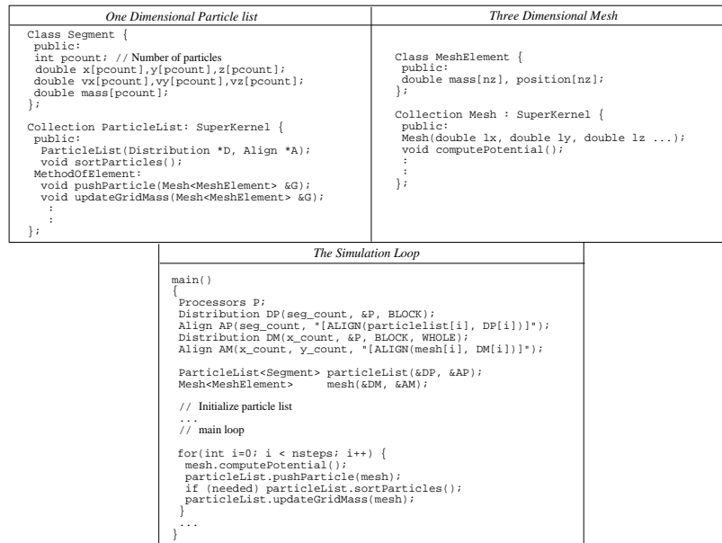
Figure 4: THE 1D PARTICLE LIST AND THE 3D MESH are the primary distributed data structures in the particle mesh code. The one dimensional particle list comprises of segments and each segment has several particles in it. For each particle the position ( i.e. , x , y and z co-ordinates), velocities ( i.e. , velocities in the x , y , and z directions v_x , v_y , v_z ), and mass ( mass ) are stored. The three dimensional mesh is logically a three dimensional array of mesh points each containing the value of density and position.
