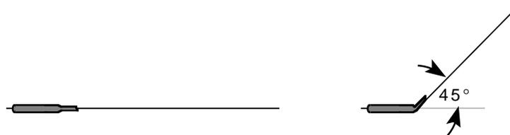
Figure 38. Bending the body crimp
