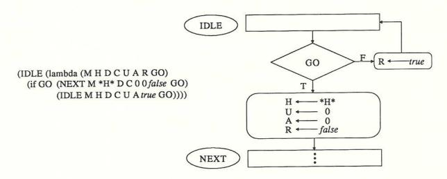
U, A, and R are updated with values \*H\*, 0, 0, and false, respectively, and NEXT becomes the new control-point. If GO is false, then R is loaded with true and the control-point does not change. ASM diagrams are used to illustrate the effect of control transformations discussed later.
