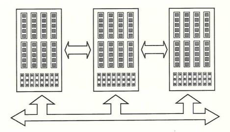
A collector for a 24-bit address space requires three identical chips, only one of whose tag fields is used, and an external PLD controller. The three-chip decomposition was done to save prototyping costs by using the smallest appropriate chip frame. It does not result in a viable realization. A distribution of arithmetic propagates carries across chip boundaries; hence, the speed of the circuit is below what is needed to drive a conventional memory at reasonable rates.
