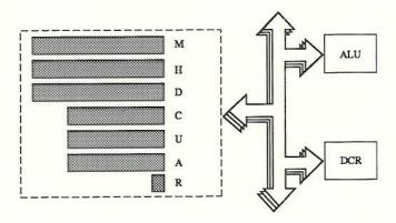
The serialization transformations discussed in the previous section have the effect of reducing the number of physical paths needed. The degree of serialization is a matter of choice. In this instance, it is carried to the point of a conventional organization, centered about a single memory channel.
