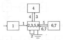
The edges  $e_1$ ,  $e_3$ ,  $e_5$  form a spanning tree, giving the fundamental cycles  $e_0:e_1$ ;  $e_2:$ ;  $e_4:e_3$ ;  $e_6:e_5$ ;  $e_7:e_5$ . This gives the independent flow equations  $E_1=E_0=1$ ,  $E_3=E_4$ ,  $E_5=E_6+E_7$ .
