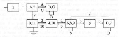
The edges  $e_1$ ,  $e_C$ ,  $e_2$ ,  $e_3$ ,  $e_4$ ,  $e_5$ ,  $e_6$  form a spanning tree, giving the fundamental cycles  $e_0: e_1, e_2; e_A: e_C; e_B:; e_D:, e_7: e_5, e_6; e_8:; e_9: e_4; e_{10}: e_3$ . This gives the independent flow equations  $E_1 = E_2 = E_0 = 1$ ,  $E_A = E_C$ ,  $E_3 = E_{10}$ ,  $E_4 = E_9, E_5 = E_6 = E_7.$
