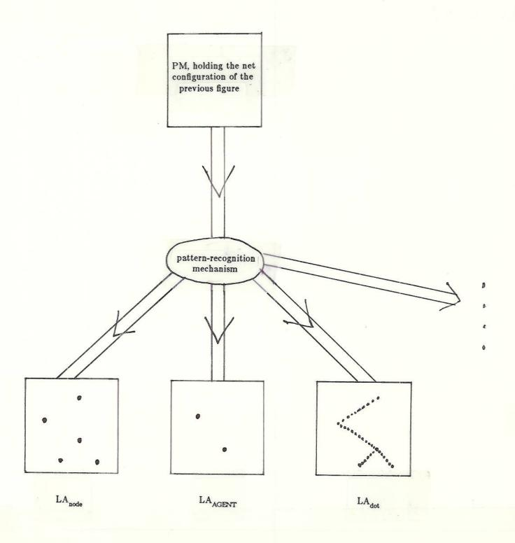
Fig. The function of the pattern-recognition mechanism. LA<sub>node</sub> is the node-pattern location array for the network configuration in Fig. 10. LA<sub>AGENT</sub> and LA<sub>dot</sub> are the AGENT-pattern and dot-pattern location arrays for that network configuration. Dots in this array boxes in the figure indicate the 1s. All the other values in the arrays are zero. Not shown are the location arrays for the node labels and for the link labels other than AGENT.
