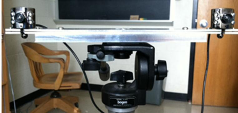
Figure 2: Our two USB cameras mounted on our custom built platform. Our camera platform can be screwed into a tripod stand using a threaded 1/4-20 hole. The camera lens centers are spaced 12” apart and secured rigidly in place.
