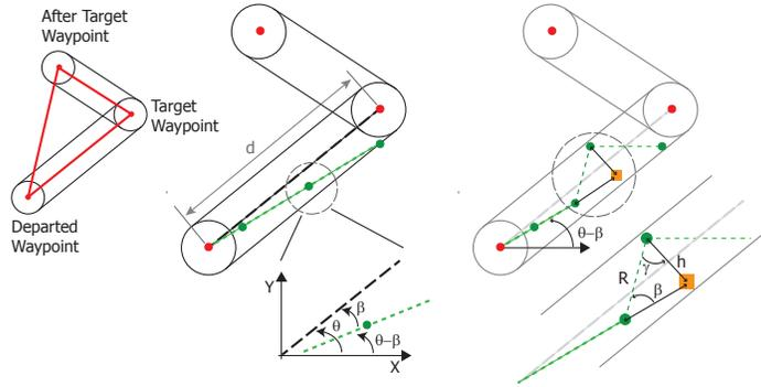
Figure 6: Schematic showing our algebraic calculations of obstacle avoidance.
