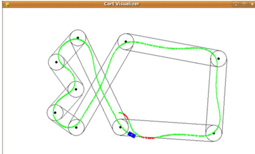
Figure 3: Simulation results using the Cart Visualizer. As in Figure 2, eight additional waypoints were included spaced equally between 10% and 80% of the distance between original waypoints. The added waypoints are not shown here, but have an LBO of 1.5 meters, versus the original waypoints which have an LBO of 2.5 meters. The cart stays fully within the corridors, the only exception being when it first starts navigating the course.
