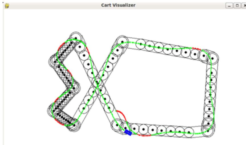
Figure 2: Simulation results from the implemented path planning routine. In this example simulation we added eight additional waypoints between each pair of waypoints. An additional waypoint was added at 10% - 80% in 10% intervals of the distance between each pair of waypoints. Each additional waypoint has the same LBO as the waypoints provided.
