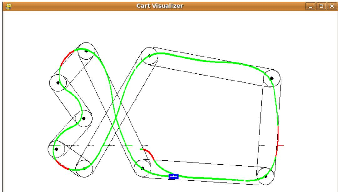
Figure 5: Telemetry data showing latitude and longitude of the cart. The cart navigated the course and passed within the LBO of each of the nine predefined waypoints and the additional waypoints introduced for path planning. Each waypoint, and its corresponding LBO, is colored to make them easier to identify.
