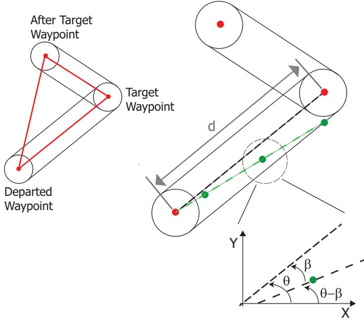
Figure 1: Schematic illustrating additional waypoints for path planning. Red dots represent the original predefined waypoints. Green dots represent added waypoints. shown too are the center line down the corridor center (black dashed line) and the line connecting the additional waypoints (green dashed line).
