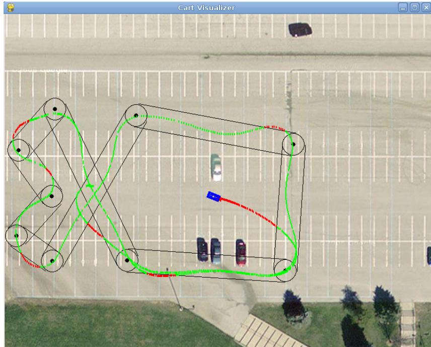
Figure 4: Mixed results during field testing of our initial path planning program. the cart is moving in a counter clockwise direction. The movements toward the AWP positioned at  $(0.9 \times d)$  were clearly deviating from our design. AWP at these positions are just before a predefined waypoint.  $d$  represents the distance between each pair of waypoints.
