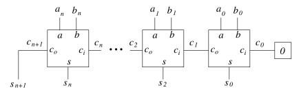
The carry bit  $c_{i+1}$  is 1 whenever two or more of the inputs are 1s, that is,
