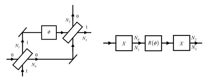
FIG. 2: Left: Diagram of the Mach-Zehnder interferometer, consisting of two beam splitters, two mirrors, and a device that changes the phase of the light wave by  $\phi$ . Right: Diagram of the equivalent quantum network.
