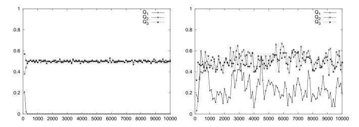
FIG. 8: Event-by-event simulation of Shor's quantum algorithm for factoring the integer N = 15, using the value a = 7 (see Section II E). Each data point represents the average of 100 output events. The parameter that controls the learning process of the DLMs is  $\alpha = 0.99$ . Left: Deterministic simulation employing DLMs. Right: Stochastic simulation employing SLMs.
