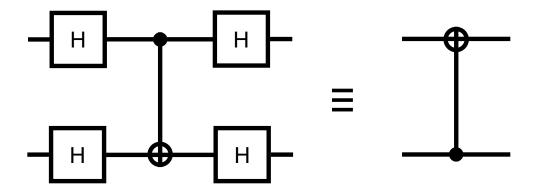
FIG. 3: Quantum circuit representation of a CNOT gate where the second (bottom) qubit acts as control qubit and the first (top) qubit is the target qubit.
