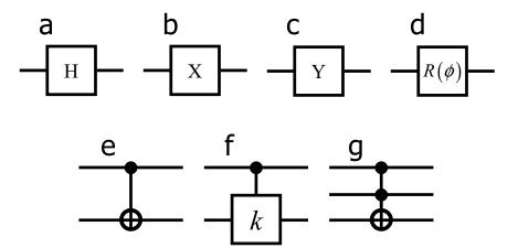
FIG. 1: Graphical representation of some of the basic gates used in quantum computation; (a) Hadamard gate; (b) Rotation by  $\pi/2$  about the *x*-axis; (c) Rotation by  $\pi/2$  about the *y*-axis; (d) Single qubit phase shift by  $\phi$ ; (e) CNOT gate; (f) Controlled phase shift by  $\phi = \pi/k$ ; (g) Toffoli gate. The horizontal lines denote the qubits involved in the quantum operations. The dots and crosses denote the control and target qubits, respectively.
