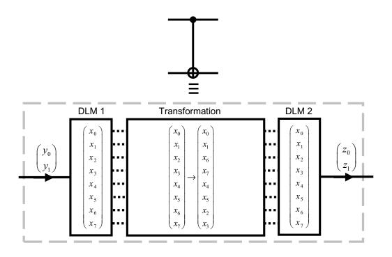
FIG. 7: Diagram of a DLM-based processor that simulates a CNOT gate on an event-by-event basis.
