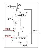
The pushbuttons and switches are asynchronous, of course, but our architecture sketch (and later our control diagram) refer to synchronous inputs such as SW. Part of the work of the implementation is to synchronize these signals, but suppose, for the moment that external inputs have been synchronized.
