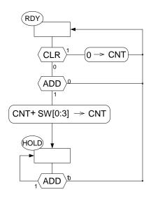
At this point, one should stop to analyze pathelogical cases arising from our algorithm, such as how it behaves when both buttons are pushed, and so forth. Tracing the paths through the decision blocks, there do not appear
