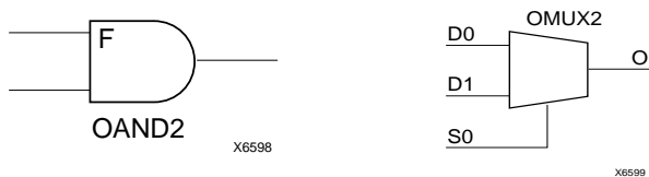
Figure 20: AND & MUX Symbols in XC4000X IOB
