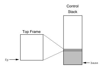
**Figure 2.** The traditional stack model provides the least expensive frame linkage. Since frames are physically adjacent, frame links can be maintained by simple register adjustments. However, since continuation operations require time proportional to the size of the active portion of the stack, the amount of time required is effectively unbounded.
