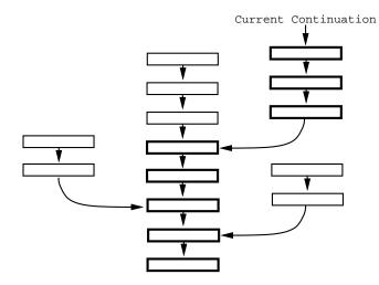
**Figure 1.** The heap model provides the simplest method for supporting constant-time continuation operations. An activation record is allocated in the heap and linked to the current activation record before a call is made. The called procedure uses the link to restore the old frame pointer before returning. Continuation operations involve saving or restoring a pointer to the current frame.
