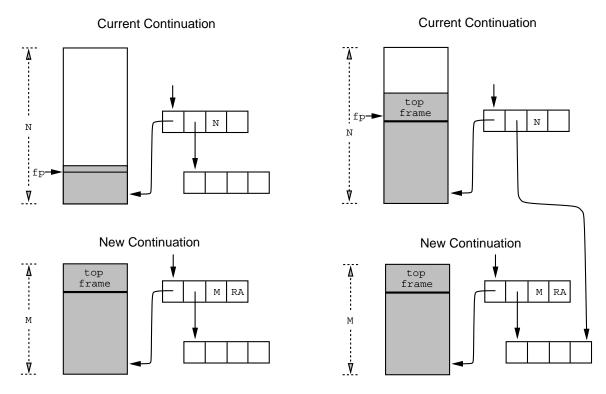
**Figure 6.** When a continuation is reinstated, the contents of the stack segment of the continuation is copied into the current stack segment. If the size of the stack segment is greater than a predetermined limit, the segment is first split into two segments (see Figure 7). If the current stack segment is not large enough to hold the contents of the reinstated stack segment, a new stack segment is allocated.
