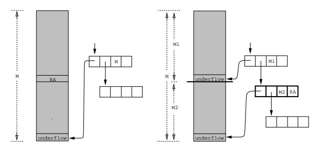
Figure 7. Large stack segments must be split before being reinstated. A splitting point is found by walking the stack to find the frame that gives the largest value for M1 without exceeding the predetermined limit on copying. The return address at the splitting point is stored in a new stack record and the address of an underflow handler is stored in its place.
