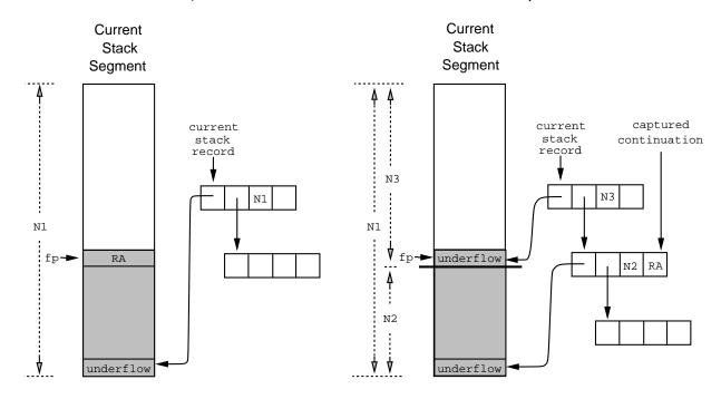
Figure 5. Capturing a continuation is a constant-time operation with the segmented stack model. The current stack segment is divided into two segments at the top frame. The bottom segment is the stack segment for the captured continuation, and the top segment becomes the current stack segment.
