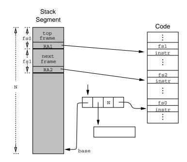
**Figure 4.** Walking backwards through a stack segment is straightforward. The return address field of a continuation stack record points to an instruction in the code stream, which is preceded by a data word containing the frame size. This frame size is used to to find the base of the top frame, where its return address is stored. This return address is used to find the frame size of the next frame down, which is used to find the next return address, *etc.*
