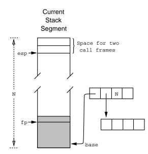
Figure 8. The end-of-stack pointer, *esp*, always points to a region before the actual end of the stack. This region must contain enough space for two call frames. Reserving room for two frames simplifies the overflow check for procedures that make recursive (non-tail) calls and eliminates the overflow check for procedures that do not make recursive calls.
